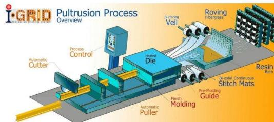
After the composite comes out of the die, it is allowed to post-cure while being pulled to the automatic saw where it will be cut to designed lengths.
